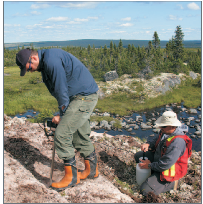
Aurora's Exploration Manager, Steve Barrett, uses a packsack drill to collect core samples from a new showing, near the White Bear prospect, during the 2009 work program. Paul McNeill, Aurora's Vice President of Exploration, is at right. We had a very successful program, discovering many new showings and three new zones of mineralization slated for further work.
